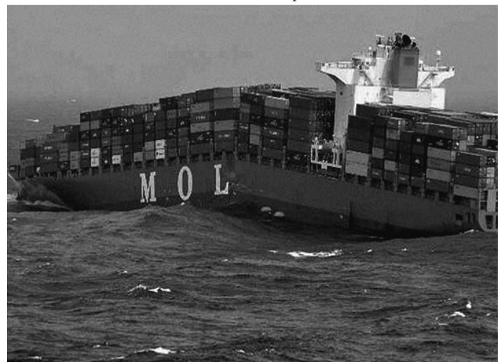
The MV MOL Comfort about to break into two sections
